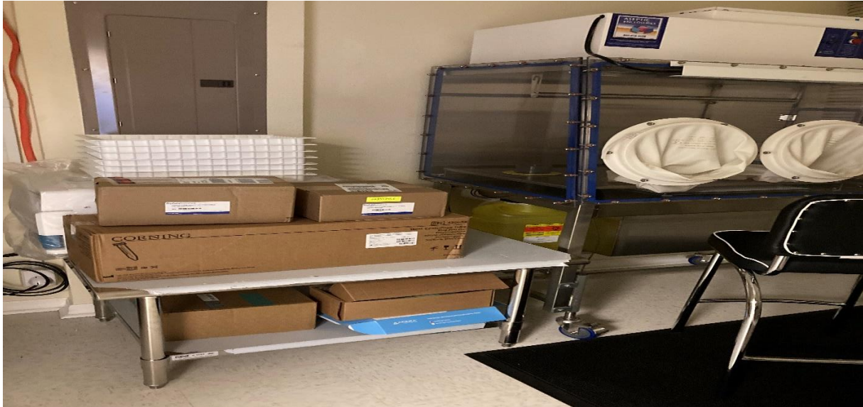
Exhibit 3 Negative pressure CACI in SCA uncertified and surrounded with cardboard.
