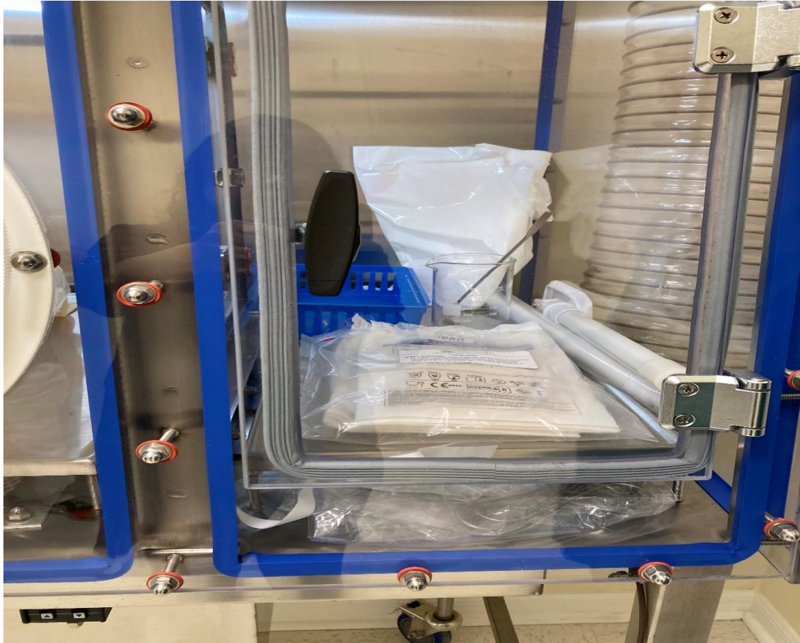
Exhibit 7 Cluttered Antechamber where Active Pharmaceutical Ingredient Powder is weighed in an uncertified hood.
